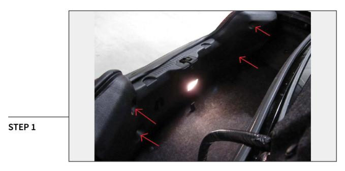
Open the trunk and remove the plastic trunk liner by removing the (4) clips securing it to the body.
