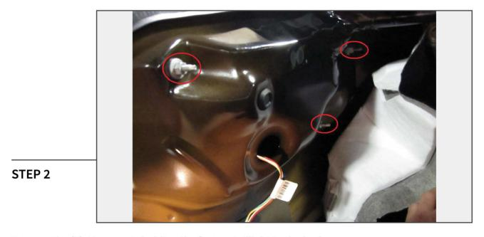
Remove the (3) 11mm nuts holding the factory taillight to the body.
